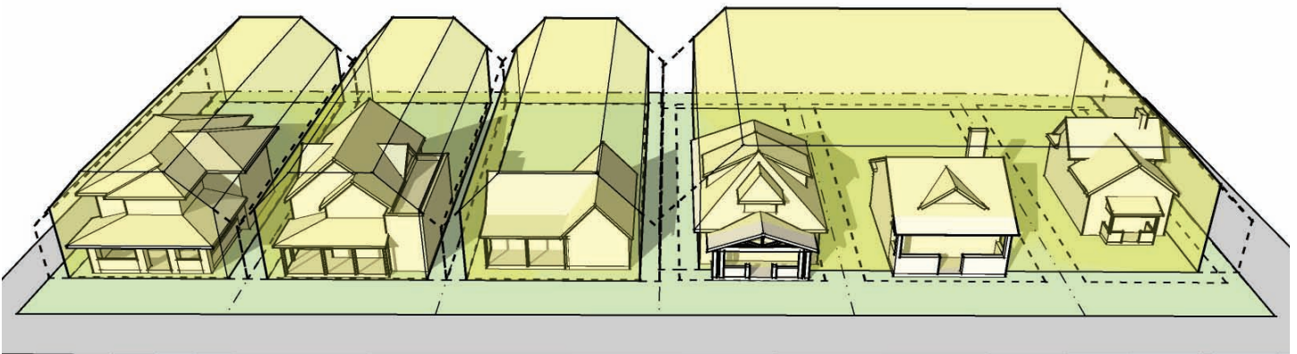
Figure 1.12c: A half block on 11th Street between Maple and Illinois, zoned as R3. This image shows the permitted envelope if three of the lots were to be consolidated for townhouses.
